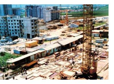
**Permanent plants** use appropriate bridge cranes, concrete plants, common equipment for concrete deposition (poker vibrators, external vibrators, vibrating plates), reinforcing sections with adequate equipment for straightening, cutting and rebar and assembly shaping, steam boiler room for steam curing of freshly set in concrete elements, workshops for equipment maintenance and the laboratory for quality control of the concrete.
