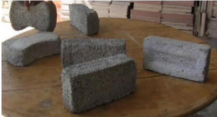
The ecological brick is made by debris of excavation (clay), remains of ground and crushed construction, integrated by a natural additive, a mixture of water with [Nopal mucilage](#). In addition, for drying the brick solar energy is used instead of the traditional cooking method for the bricks.
