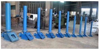
without external energy like electricity or fuel and only on the power/energy of water. It needs free flowing water, like springs, streams, creeks and rivers. The falling water contains the energy to pump the water up and it is converted in the ram system into pressure.
