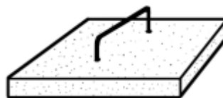
Concrete lid with metal handle
