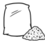
About 3 1/4 litres or 3 quarts of washed separation gravel
