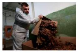
Releaf Paper developed its own patented technology of processing fallen leaves info fibers. Using combination of mechanical, thermal and chemical treatment, they not only dispose green wastes, but also ensure source of sustainable raw-materials for paper & packaging industries. The benefits of the production process are the following:
