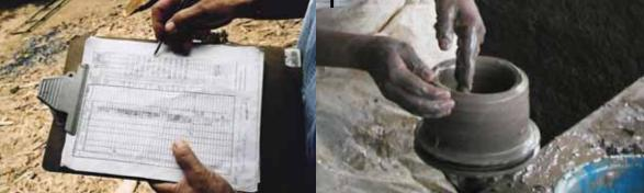
**FILTRÓN is** a very inexpensive product. The filter can be made by local potters using local materials, with no need for electricity or advanced technology. It consists of a mixture of 50% red clay and 50% sawdust, or similar organic material such as rice husk or coffee husk, depending on locally available material. Water is added to the mixture, which is then placed into a mould. This is then pressed using a truck jack, which is something that can be easily found.
